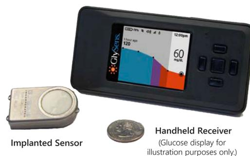
**Figure 1. The Model 100 ICGM Sensor with the system receiver.** The sensor is fully implantable and requires no on-the-skin or body-worn components. The handheld receiver displays blood glucose trends and provides alerts and glucose history.
