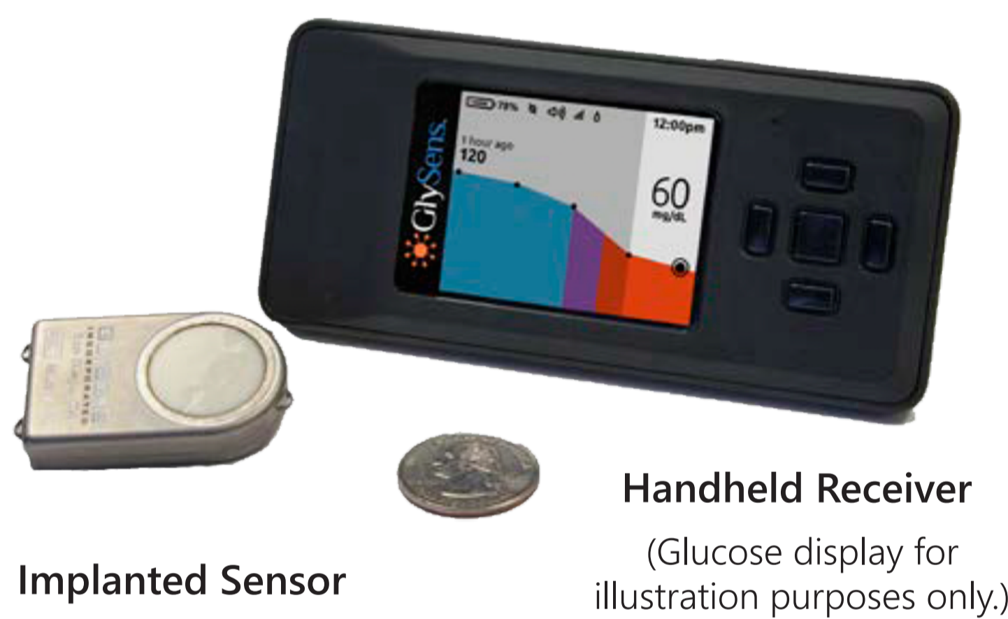
Figure 1. The Model 100 ICGM Sensor with the system receiver. The sensor is fully implantable and requires no on-the-skin or body-worn components. The handheld receiver displays blood glucose trends and provides alerts and glucose history.
