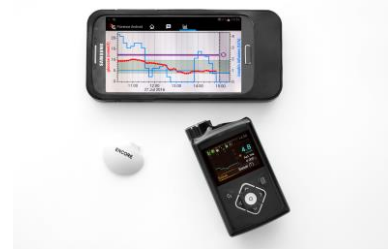
Figure 2. FlorenceM closed-loop system
