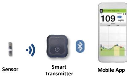
The Eversense CGM System utilizes a long-term implantable glucose sensor powered by an external, wearable smart transmitter through a wireless inductive link. The sensor is fluorescence-based and developed for subcutaneous insertion in the upper arm. The smart transmitter wirelessly communicates with the mobile app to display real-time glucose readings, trends, and alerts.
