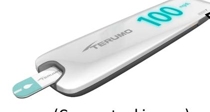
High accuracy: *Within*  $\pm 5\%$ (95% of all values) Short measurement time: Within 5 seconds Easy-to-use: Easy to handle, Calibration less Reasonable price
