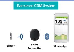
The Eversense CGM System utilizes a long-term implantable glucose sensor powered by an external, wearable smart transmitter through a wireless inductive link. The sensor is fluorescence-based and developed for subcutaneous insertion in the upper arm. The smart transmitter wirelessly communicates with the mobile app to display real-time glucose readings, trends, and alerts.
